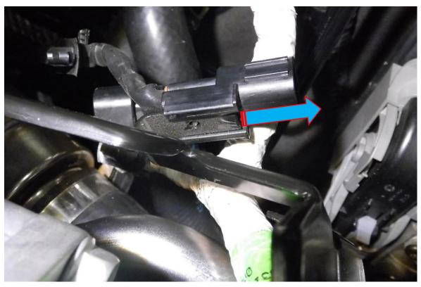
10. Using the supplied cable tie with the FMTIA11 kit, secure the Lambda loom to the coolant hose but not too tight.
