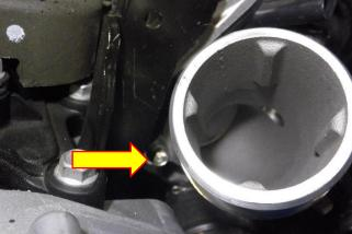
8. <u>IMPORTANT</u> Before installing the Forge Motorsport turbo adaptor, make sure the original O-ring is seated correctly into the turbo.
