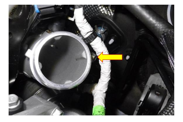
6. Using long nose plyers loosen the hose clamp to allow the removal of the oil breather pipe attached to the turbo adaptor.
