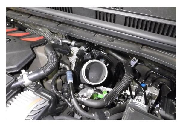
**13**. Re-attach the oil breather hose to the Forge Motorsport turbo adaptor and plug the wiring loom back into the turbo actuator.
